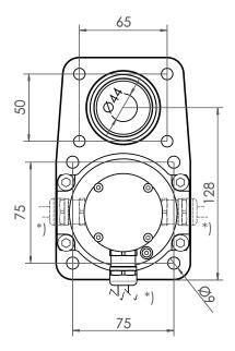
\*) Three different orientations possible for the cable outlet
