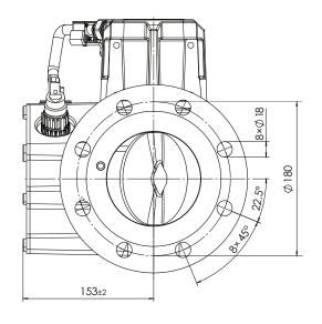
Flange according to DIN 1092-1 DN100 / PN16
