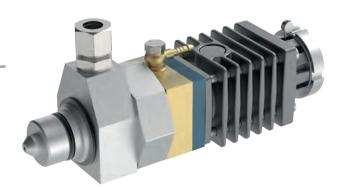
Differing to RPLV-1S the 2S-version additionally offers the important limp-home function. After opening due to overpressure RPLV-2S works as a rail pressure control valve and keeps up some holding pressure under any system conditions even without risk of overheating. This provides high reliability and ensures engine running.
