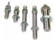
HEINZMANN inductive speed sensors are available with metric or inch threading. Sensors have IP55 protection rating and are designed for frequencies from 50 to 12,000 Hz and air gap range 0.5 - 2.5 mm.
