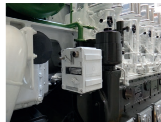
HEINZMANN ELEKTRA Gas Metering Unit and Actuator mounted on ABC Dual-Fuel Engine
