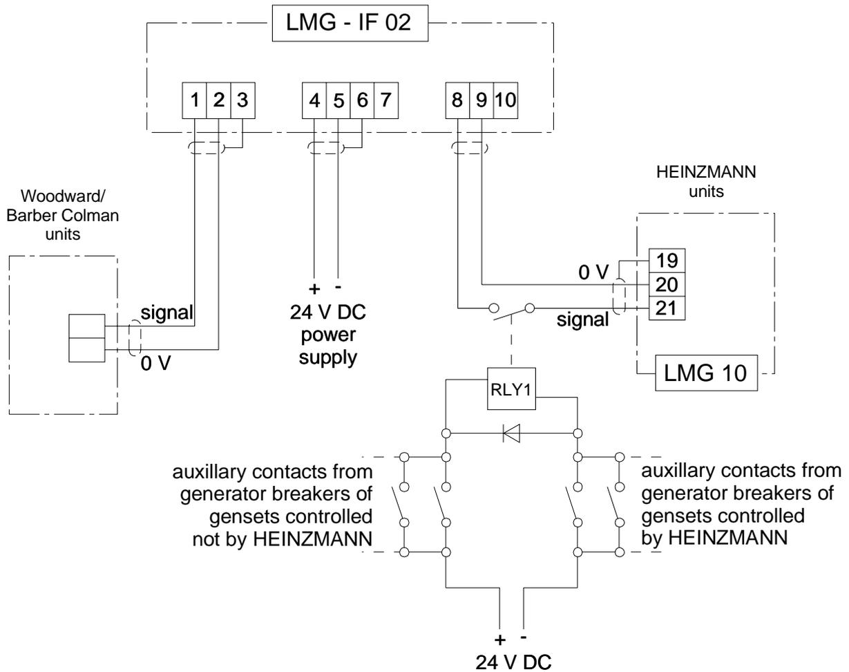
Figure 2: Electrical Connection of LMG – IF
